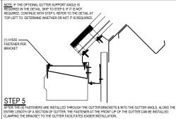
NOTE: IF THE OPTIONAL GUITER SUPPORT ANGLE IS REQUIRED. IT CAN BE INSTALLED AT THIS TIME. THE FASTENER AT THE FRONT UP OF THE GUITTER MULL GO THROUGH THE GUITTER, GUITER SUPPORT ANGLE, AND THE GUITTER BRACKET.
